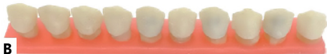
Figure 3. Digital wax-up (Milling) and conventional casting. A, 10 digital wax patterns by print-milling method on 10 resin dies. B, 10 pieces of lithium disilicate coating (IPS Emax press) obtained by milling the wax pattern on 10 pieces of resin dies.
