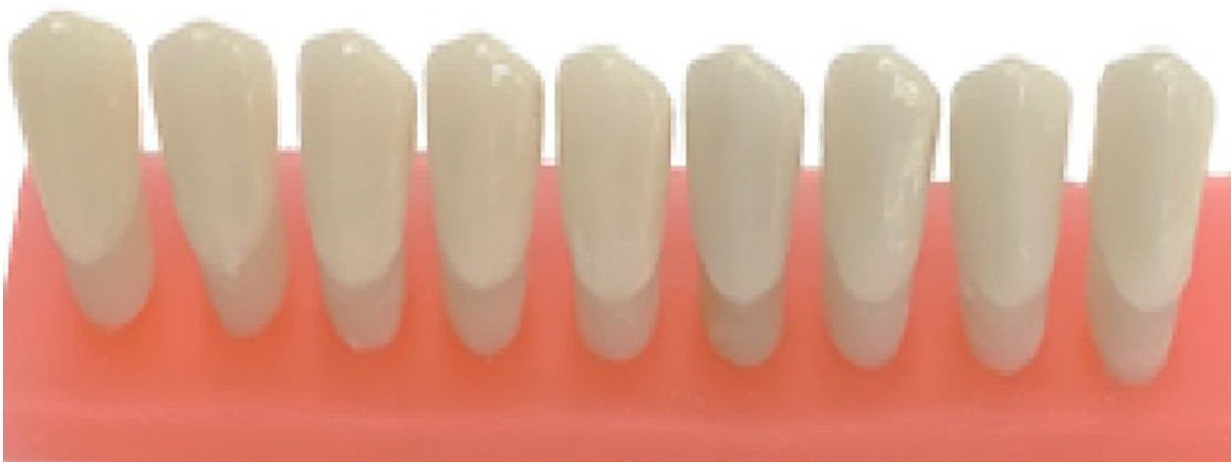
Figure 4. Fully Digital (Milling). 10 pieces of lithium disilicate crowns (IPS Emax CAD) obtained by CAD/CAM method on 10 pieces of resin dies.
