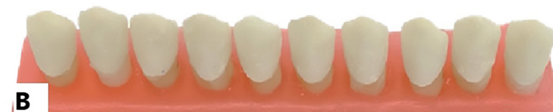
Figure 2. Digital wax-up (3D Printer) and conventional casting. A, 10 digital resin patterns by 3D printing method on 10 resin dies. B, 10 pieces of lithium disilicate crowns (IPS Emax press) obtained by 3D printing method of resin pattern on 10 pieces of resin dies.
