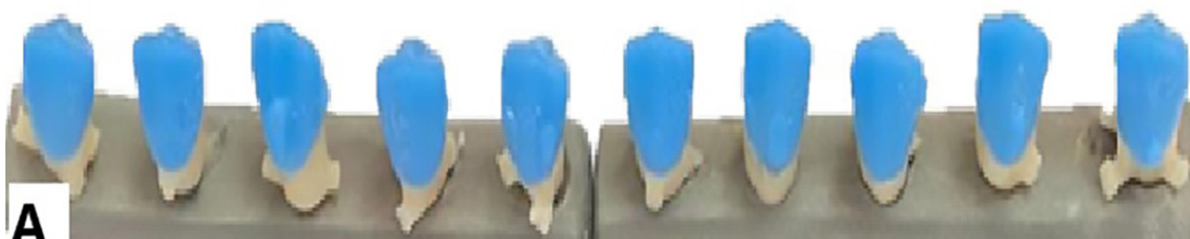
Figure 2. Digital wax-up (3D Printer) and conventional casting. A, 10 digital resin patterns by 3D printing method on 10 resin dies. B, 10 pieces of lithium disilicate crowns (IPS Emax press) obtained by 3D printing method of resin pattern on 10 pieces of resin dies.
