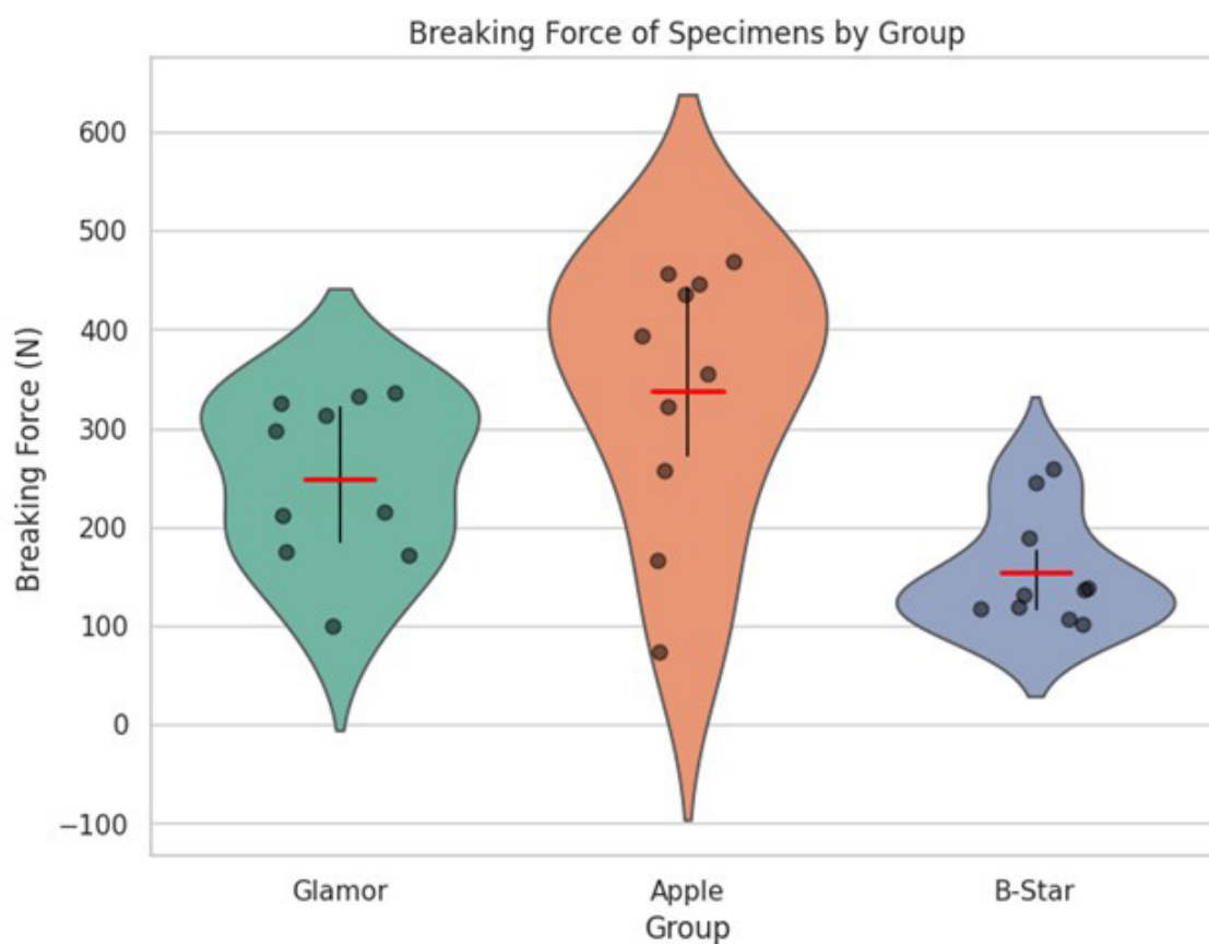
Figure 1. Breaking Force Distribution by Group; showing mean (red line), quartiles, and individual data points.
