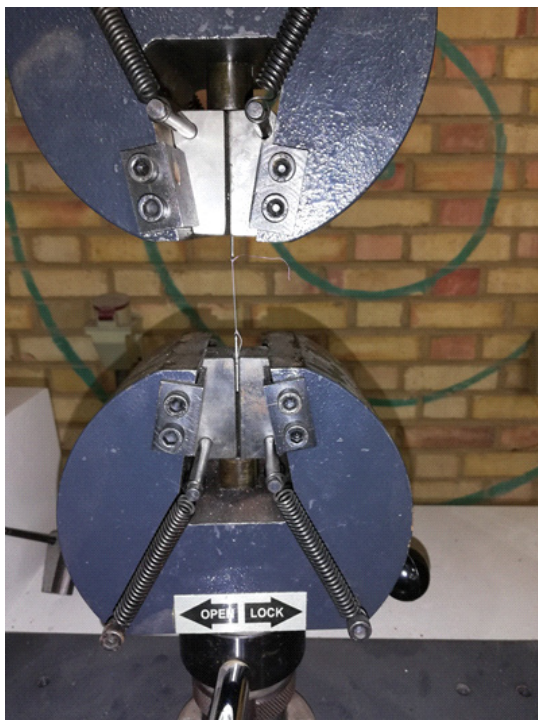
Figure 1. Tensile strength test of two types of chromic catgut and PGA by Universal Testing Machine
