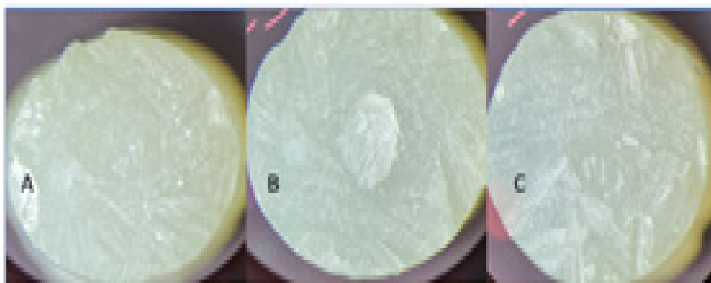
Figure 1. 50X magnification micrographs. (A) Adhesive failure; (B) mixed failure; (C) cohesive failure.
