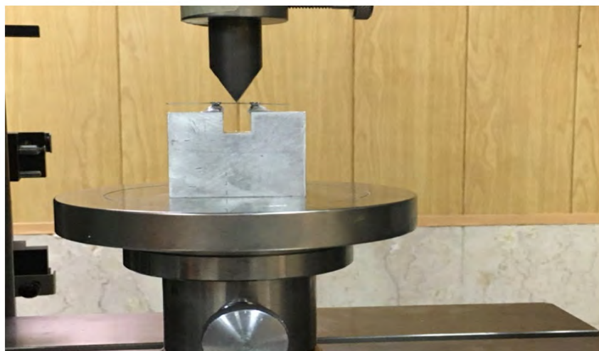
Figure 1. Loading of a wire in the three-point bending test
