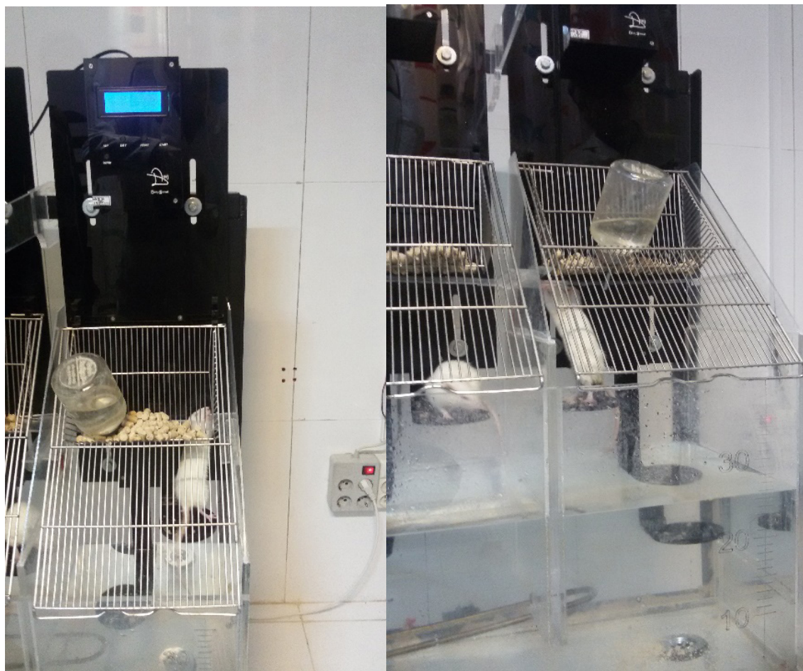
Figure 1. SD apparatus "water-box". A holding time that was considered to allow water and food intake.
